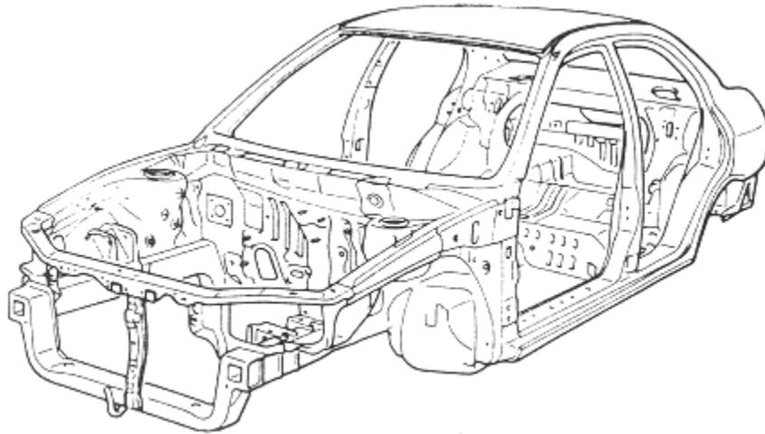
**Fig. 6.2 A Typical Body Shell Construction**
