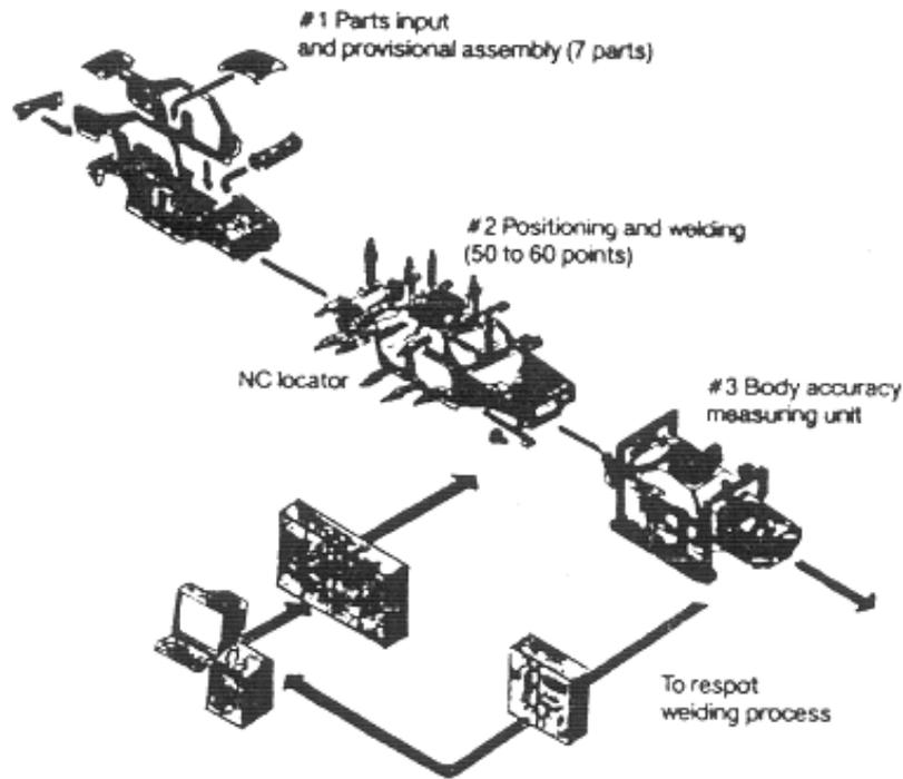
**Fig. 6.14 Stages of Nissan's Intelligent Body Assembly System**
