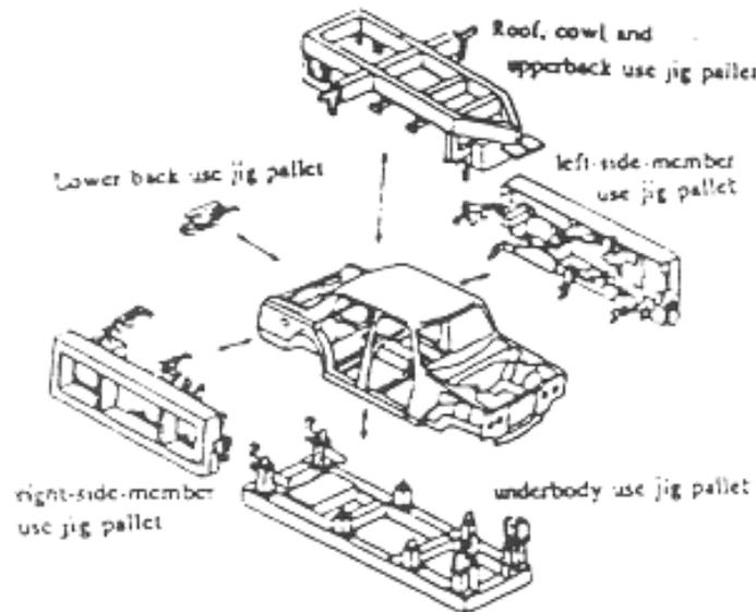
Fig. 6.13 Different Jig Pallets for Major Subassemblies
