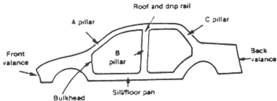
**Fig. 6.18 Possible Laser Welding Areas of Autobody**
