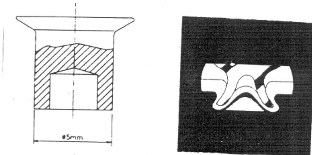
Fig. 6.19 A Self Piercing Rivet
