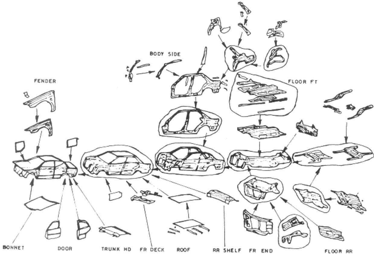
**Fig. 6.3 Sequences of Sub-Assemblies and Main Body Welding**
