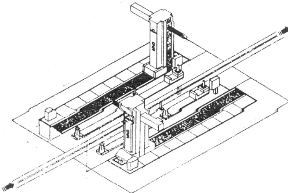
**Fig. 6.21 A Robotised Cell for Body Inspection**
