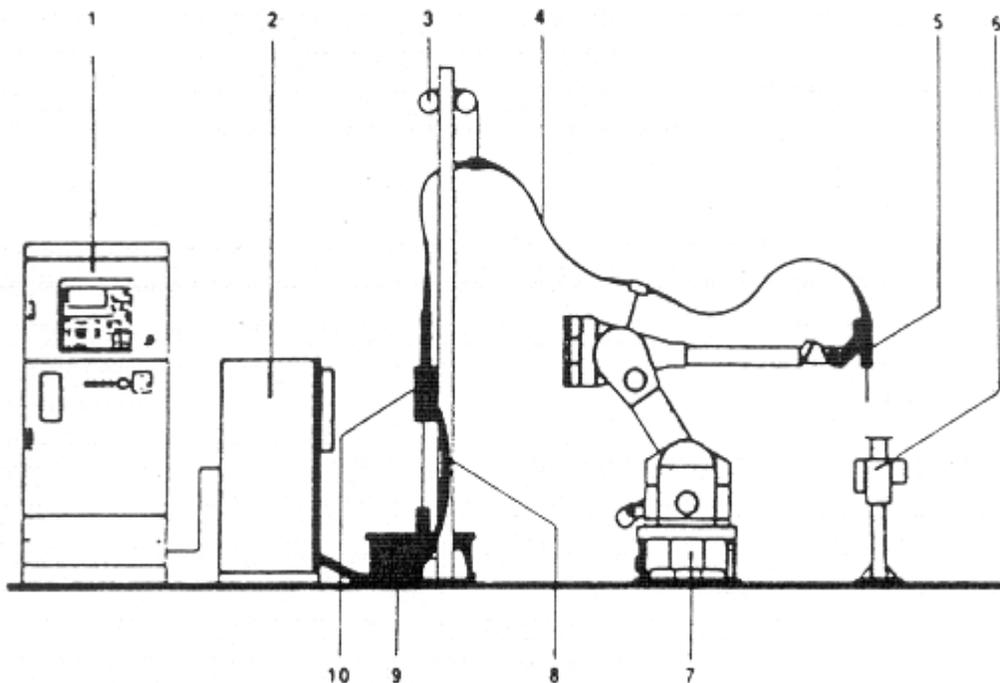
**Fig. 6.16 An Arc Welding Robot**
