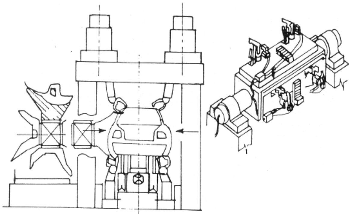
Fig. 6.7 An Improved Version of Body Framing Station
