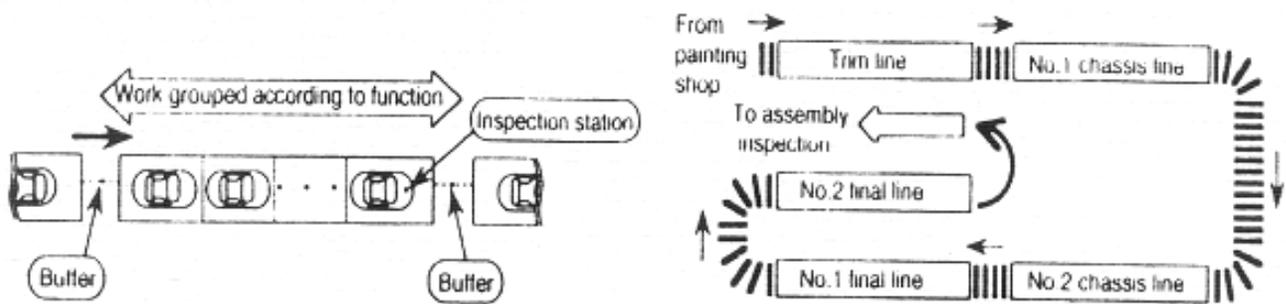
Fig. 8.12 Conventionally Long Assembly Line Divided in Small ones
