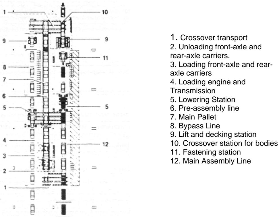
Fig. 8.8 A Chassis Assembly System
