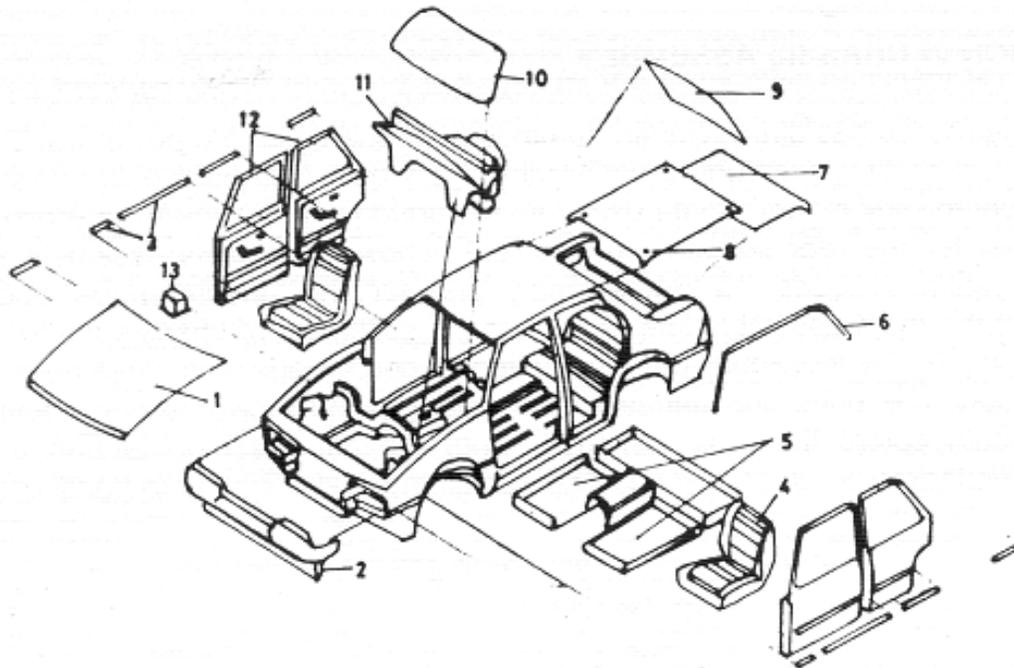
1. Hood 2. Front module 3. Guard Rail 4. Front Seat 5. Front/Rear Carpet 6. Drip Moulding 7. Trunk Lid 8. Headliner 9. Rear Lite 10. Windsheild 11. Cockpit module 12. Front/Rear door 13. Battery
