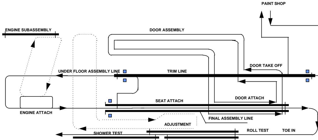
Fig. 8.1 A Typical Layout of Trim and Final Assembly
