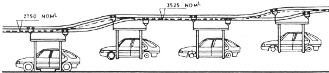
Fig. 8.5 Bodies on Tyres to Final Assembly Conveyor
