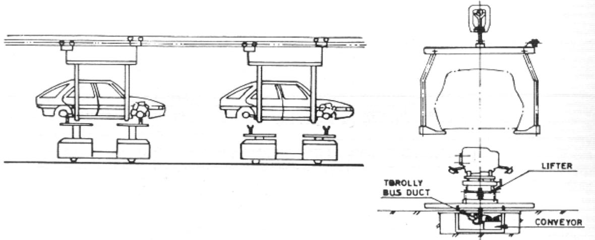
Typical arrangement of body marriage over Power Train and Rear Axle Trolleys
